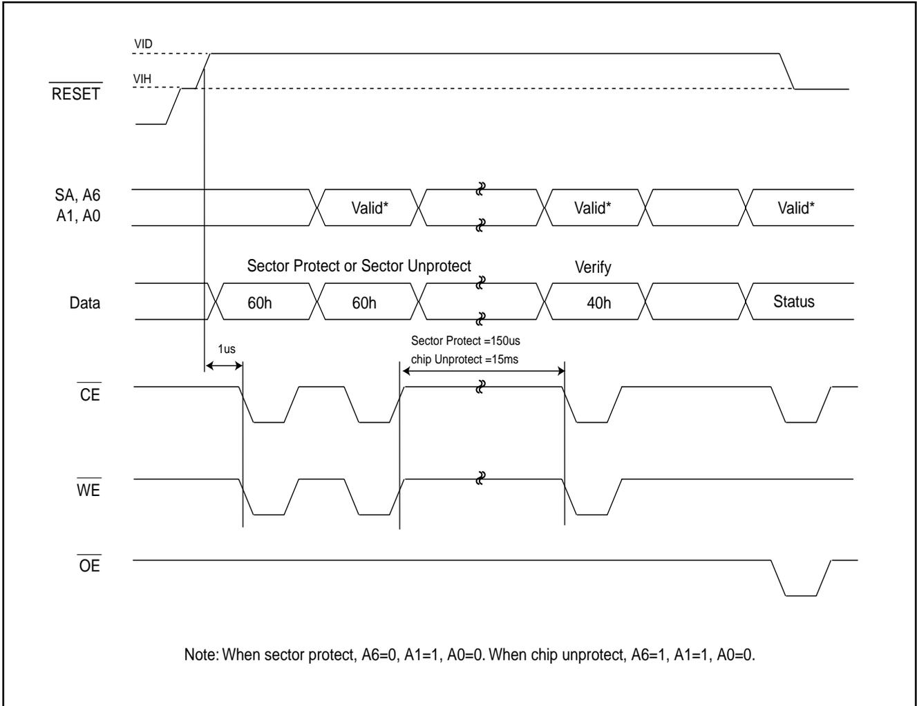
Figure 12. SECTOR PROTECT TIMING WAVEFORM (A9,  $\overline{OE}$  Control)
