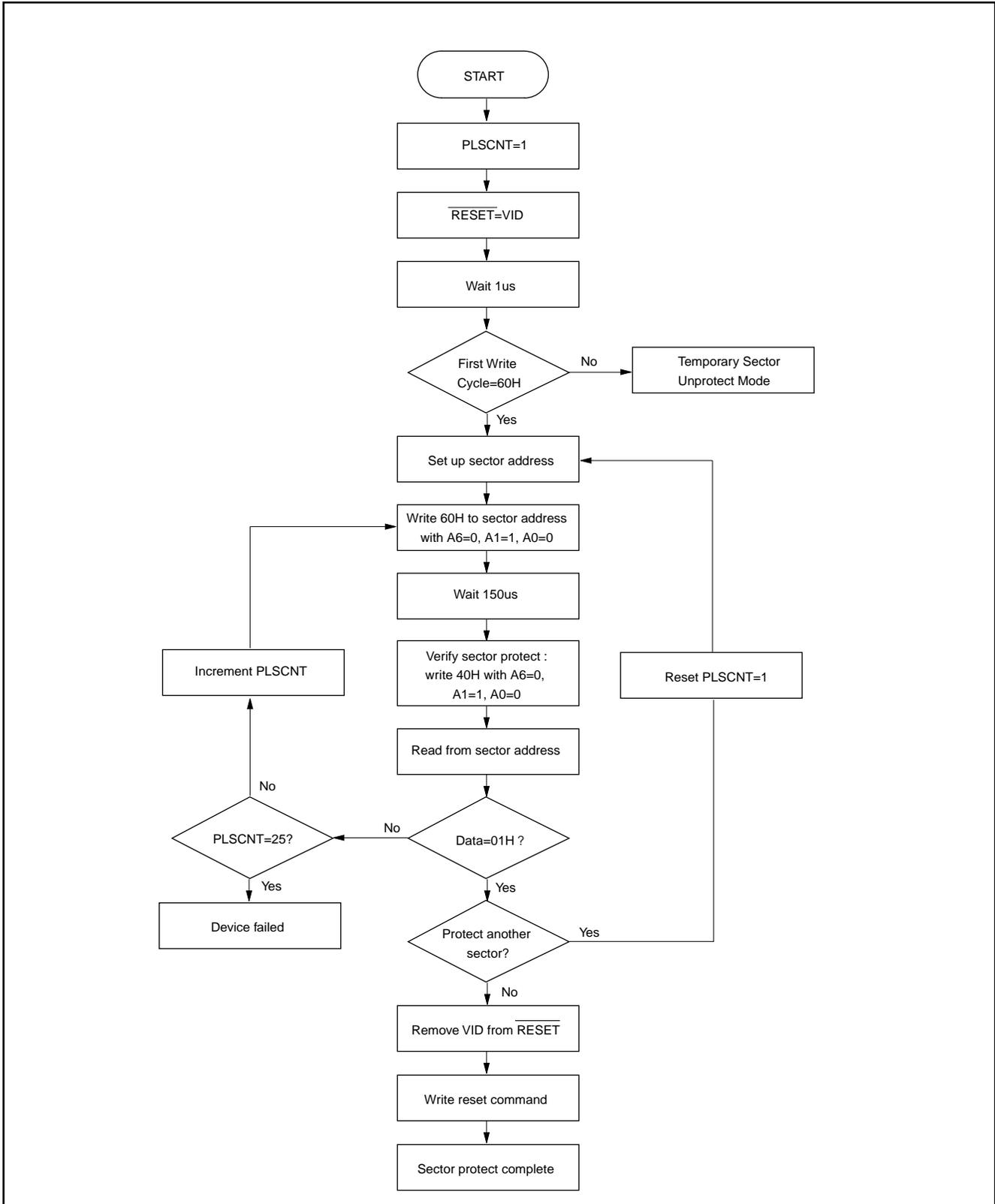
**Figure 15. IN-SYSTEM CHIP UNPROTECTION ALGORITHM WITH  $\overline{\text{RESET}}=\text{VID}$**
