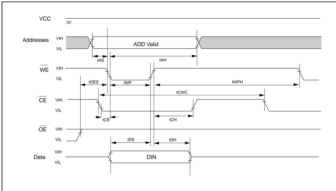
**AUTOMATIC PROGRAMMING TIMING WAVEFORM**
