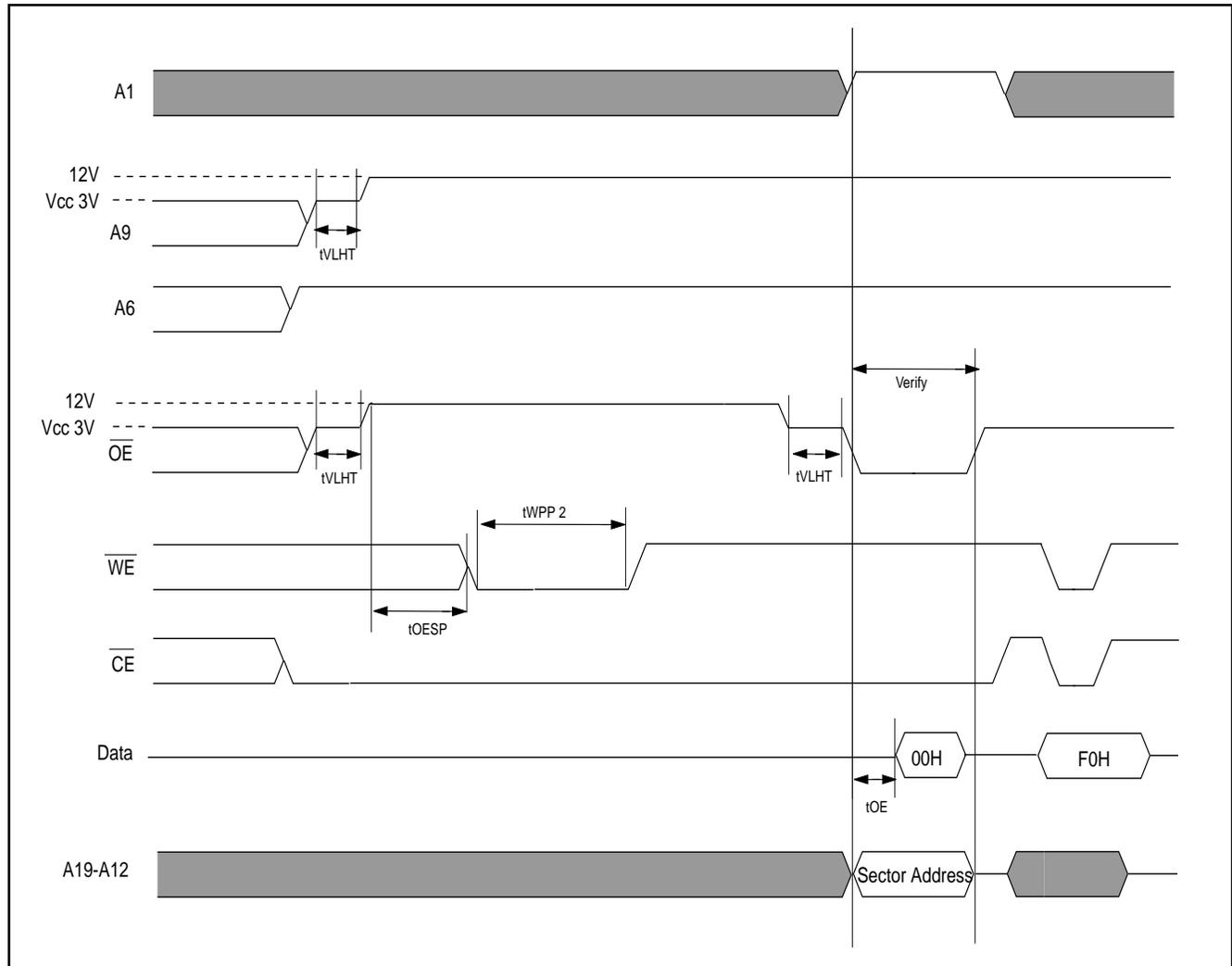
Figure 17. CHIP UNPROTECTION ALGORITHM (A9,  $\overline{OE}$  Control)
